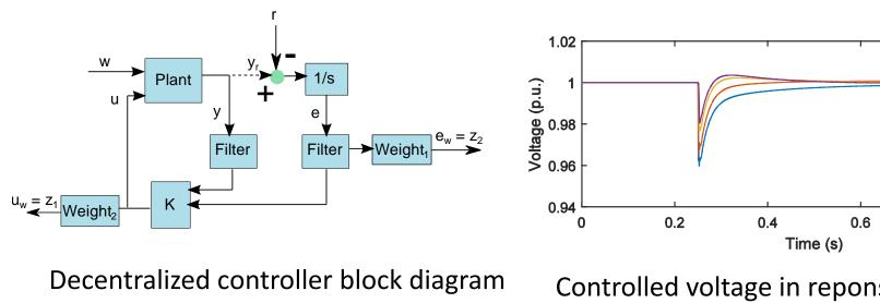
Controlled voltage in reponse to a 25% power increase (300 kW)
